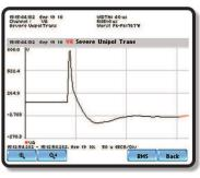
switching, lightning, transformer energization, and load shifting, are immediately characterized as impulsive or oscillatory and detailed for further analysis. Capable of capturing the complete power quality spectrum, the PowerXplorer provides scope-like display of the entire transient.
