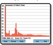
variations in performance that aggregate to effect significant long-term damage. Current harmonics generated by a source can pollute the entire power system without being affected itself. The PowerXplorer captures detailed harmonics, interharmonics and subharmonics to effectively trouble-shoot the complex problems caused by these events.
